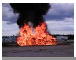
• If you must stack idle pallets higher than 6 feet, your sprinkler system should be designed specifically with ESFR heads for this type of storage.
